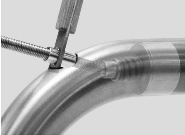
By turning the screw further, the wooden bar is pushed out of the bent tube.
