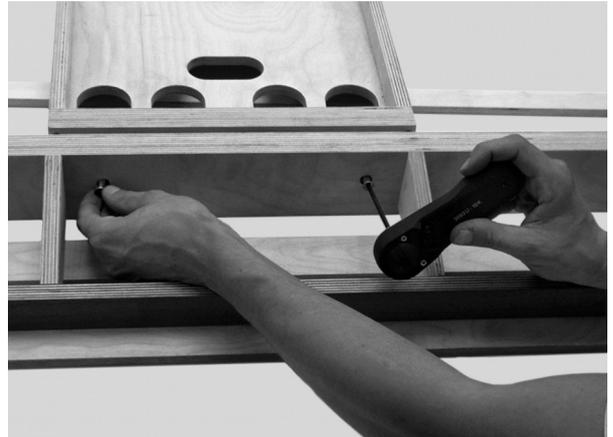
Start screwing together the cross bars against the mid rails. Use the enclosed counter sunk screws M8x60 (these are the long ones!).
