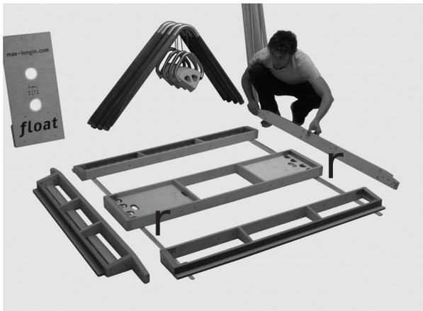
**Tip!** With two slats laid on the floor as shown above you can help yourself to meet the different heights of longitudinal supports and the crossbar (see arrows).
