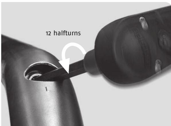
6.5 Loosen the cylinder head bolts of the spring package in all 8 bent tubes with about 6 turns.
