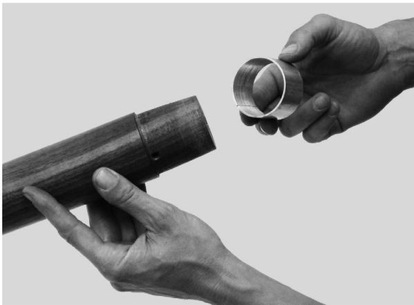
4.3 Push the sleeve only so far onto the tenon that the sleeve just sticks on the tenon.
