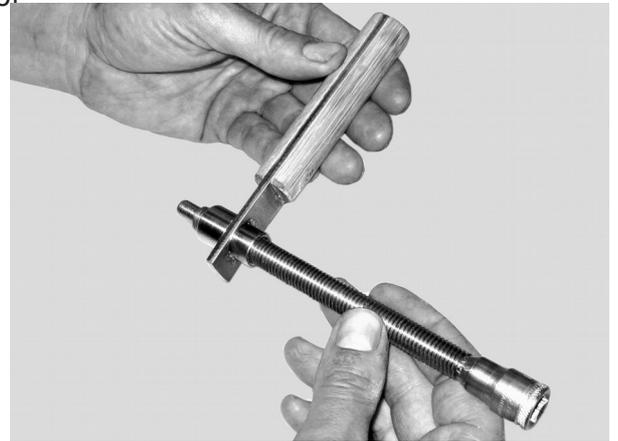
6.7 Now place the ejection-grip into the hole of the bent tube. Here the tool has to work like a hook at the edge of the hole.
