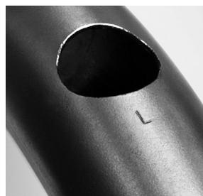
The bent tubes for the long sides don't have such a tight bent as the others and have a little marking next to the loophole "L" (- for long). The bent tubes for the short side are marked with an "S" accordingly.
