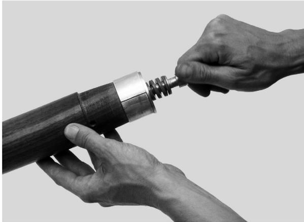
4.6 Now stick the prepared wooden bar into the bent tube.
