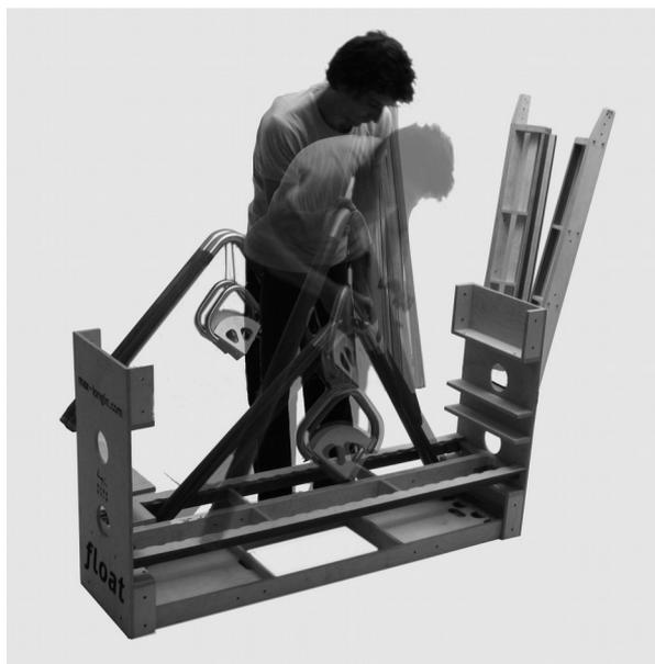
**Important!** Pay attention to the hanging corner fittings: they shouldn't knock against the wooden bars. Avoid quick and uncontrolled movements with the frame parts.
