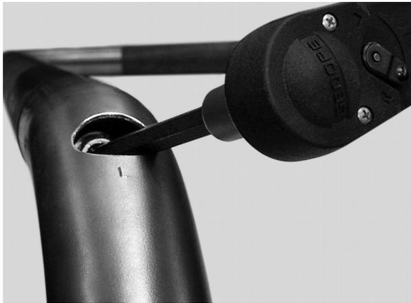
4.9 After tightening the screws, the enclosed oak cones can be pushed into the revision holes at the bent tube.
