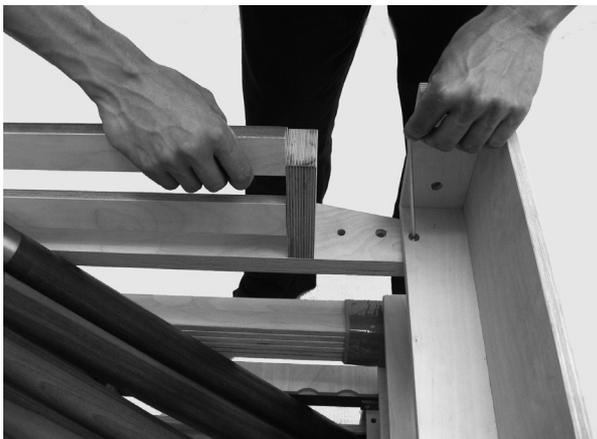
**Important!** Keep and store all the unscrewed 12 counter sunk screws M8x40 of the transport case together with the tools. You will need them later on when reassembling the bed box when you move!
