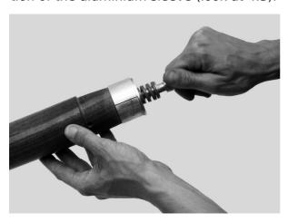
4.6 Now stick the prepared wooden bar into the bent tube.
