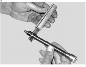
6.7 Now place the ejection-grip into the hole of the bent tube. Here the tool has to work like a hook at the edge of the hole.
