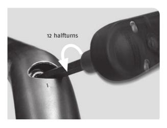
6.5 Loosen the cylinder head bolts of the spring package in all 8 bent tubes with about 6 turns.
