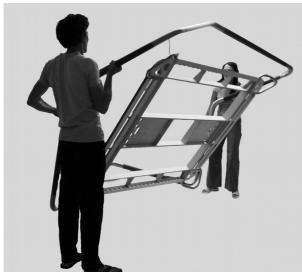
**Attention!** At a certain tilt angle during the 180 degrees turnaround the inner frame with a flip tips over into its new position. This is normal and no incorrect assemblage. Look out for a slight flip during the rotary motion and therefore slowly carry out the whole action, controlled and with a safe grip.
