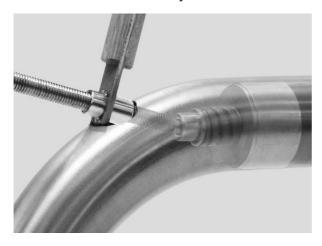
By turning the screw further, the wooden bar is pushed out of the bent tube.
