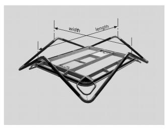
**Important!**The adherence of the mentioned dimensions between the axes is a central element for the static principle of *float*!
