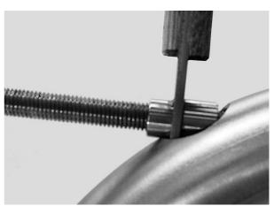
6.8 Now turn the ejection-grip screw further through the threaded sleeve. Hold the grip in the direction that the ball-shaped cone point of the screw is finally embedded into the Allen notch of the cylinder head bolt.
